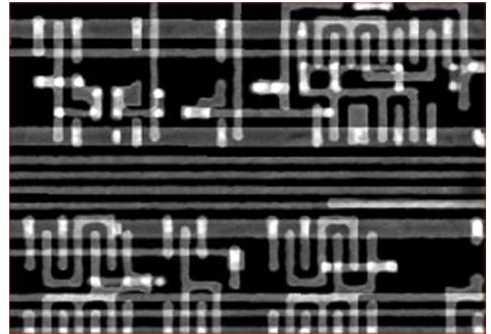
Figure 3: Overall and Close-up view showing interlayer alignment of metal and via layers.
